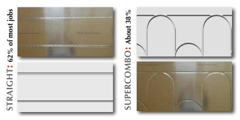
**Ecowarm Radiant Board**<sup>™</sup> is manufactured from FSC® certified plywood from sustainably managed forests. Its heavy recycled aluminum layer is bonded with a water-based VOC adhesive. Cut from standard 4′ x 8′ plywood sheets, both straight and supercombo finished board measurement is 47″ x 23.5″. Tubing (1/2″ PEX) is spaced 11.750″ on center. One-quarter radius turns measure 5.935″ from the edge.
